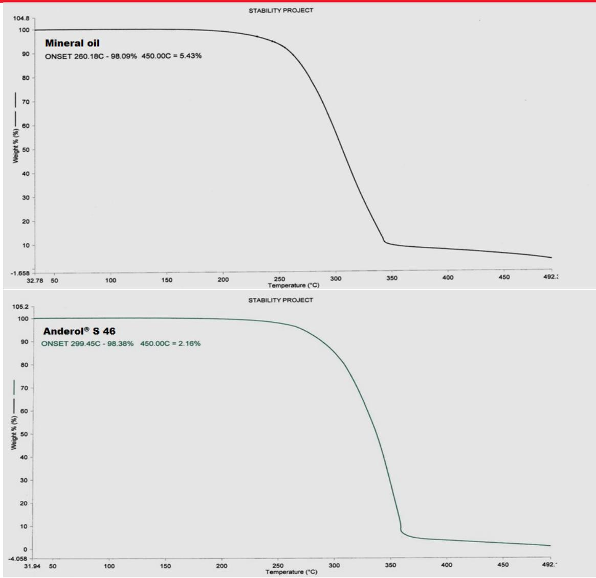
The Anderol® S range has not only a higher onset temperature which indicates a higher thermal stability, the residues are a lot less, leading to cleaner lubrication.
